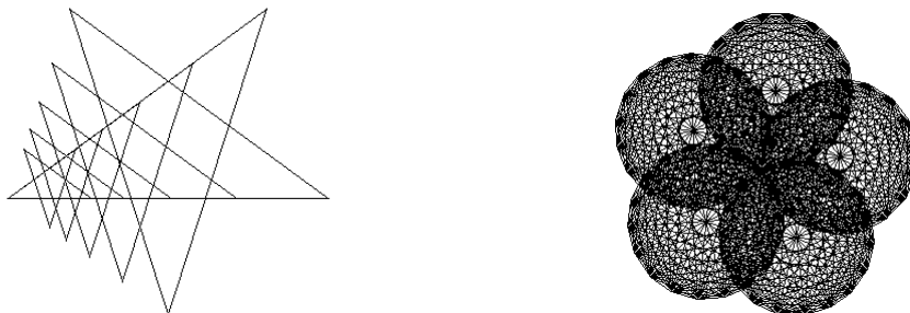
Figure 9: The effect of SCALE and SPIN. On the left, the SCALE program is applied to the turtle program for generating a star; on the right the SPIN program is applied to the turtle program for generating a rosette.
