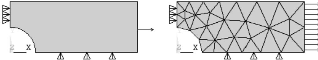
**Figure 2-13** Model with loading and displacement boundary conditions.
