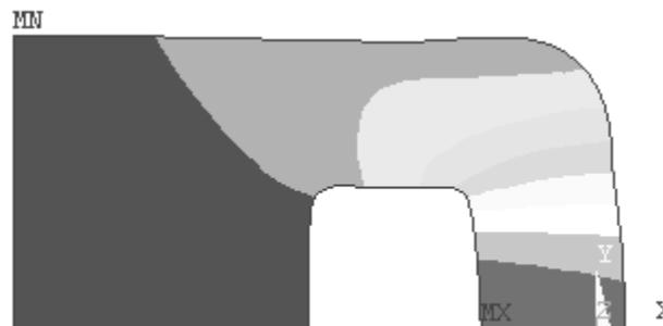
**Figure 2-31** UX displacements.
