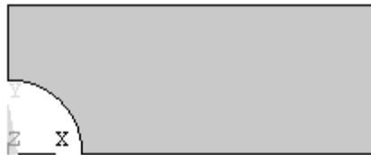
**Figure 2-11** Geometry for quadrant of plate.
