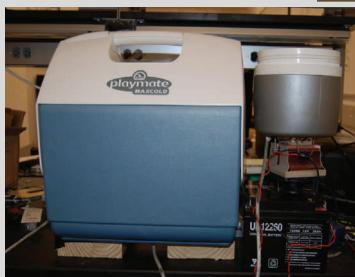
Unique design separates the cooling chamber from the medicine cooler to greatly increase efficiency and reduces the amount of time— and power— needed to keep the medicines cool.
