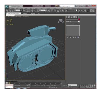
This first half is the thing that I unwrapped and readied for texturing – the texture will be mirrored on the other side, and is designed to meet up cleanly in the middle. Note that the texture doesn't actually exist yet, what I'm doing is unwrapping all the surfaces and placing them in a layout that avoids overlap and doesn't go off the edges of the texture at all. This means I can access everything and paint over it later.
