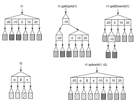
Figure 2: Intrinsic structural operations on the tree.
