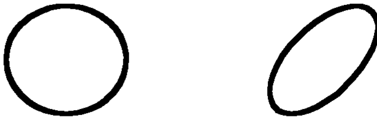
Figure 8: Scaling a circle from its center along a fixed direction generates an ellipse.
