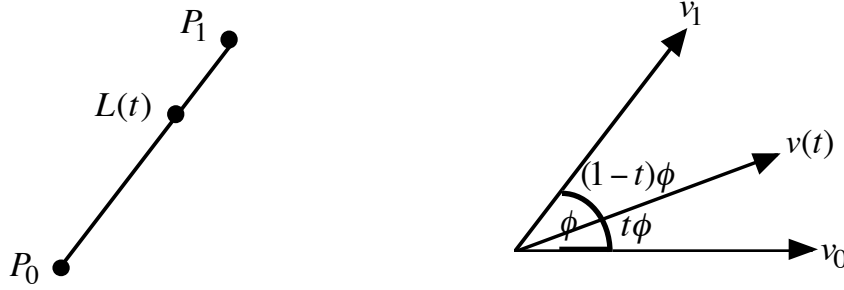
Figure 15: Linear interpolation between two points along a straight line (left), and spherical linear interpolation between two vectors along a circular arc (right).
