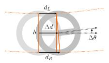
Complete this derivation. Solve for  $(x', y', \theta')$  in terms of  $(x, y, \theta)$ ,  $d_L$ ,  $d_R$ , and b. Assume the change in heading,  $\Delta \theta$ , is very small, so you can make use of the trigonometric approximation  $tan(\theta) \approx \theta$ . **Hand-in:** Your derivation.
