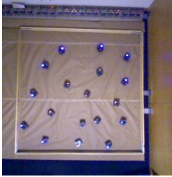
Figure 5.12: A SwarmBot experiment. Each trial started with 20 robots, but often robots would run out of batteries during a trial. These robots were not replaced until the next trial.
