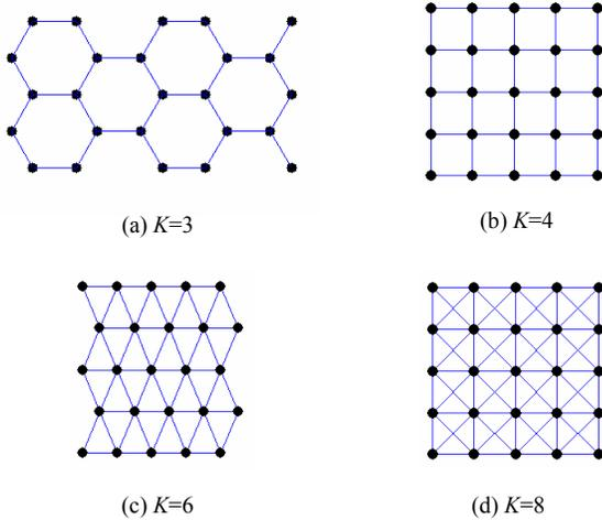
Fig. 1 Four typical topologies of mobile robot networks with  $K$ -neighbor model.
