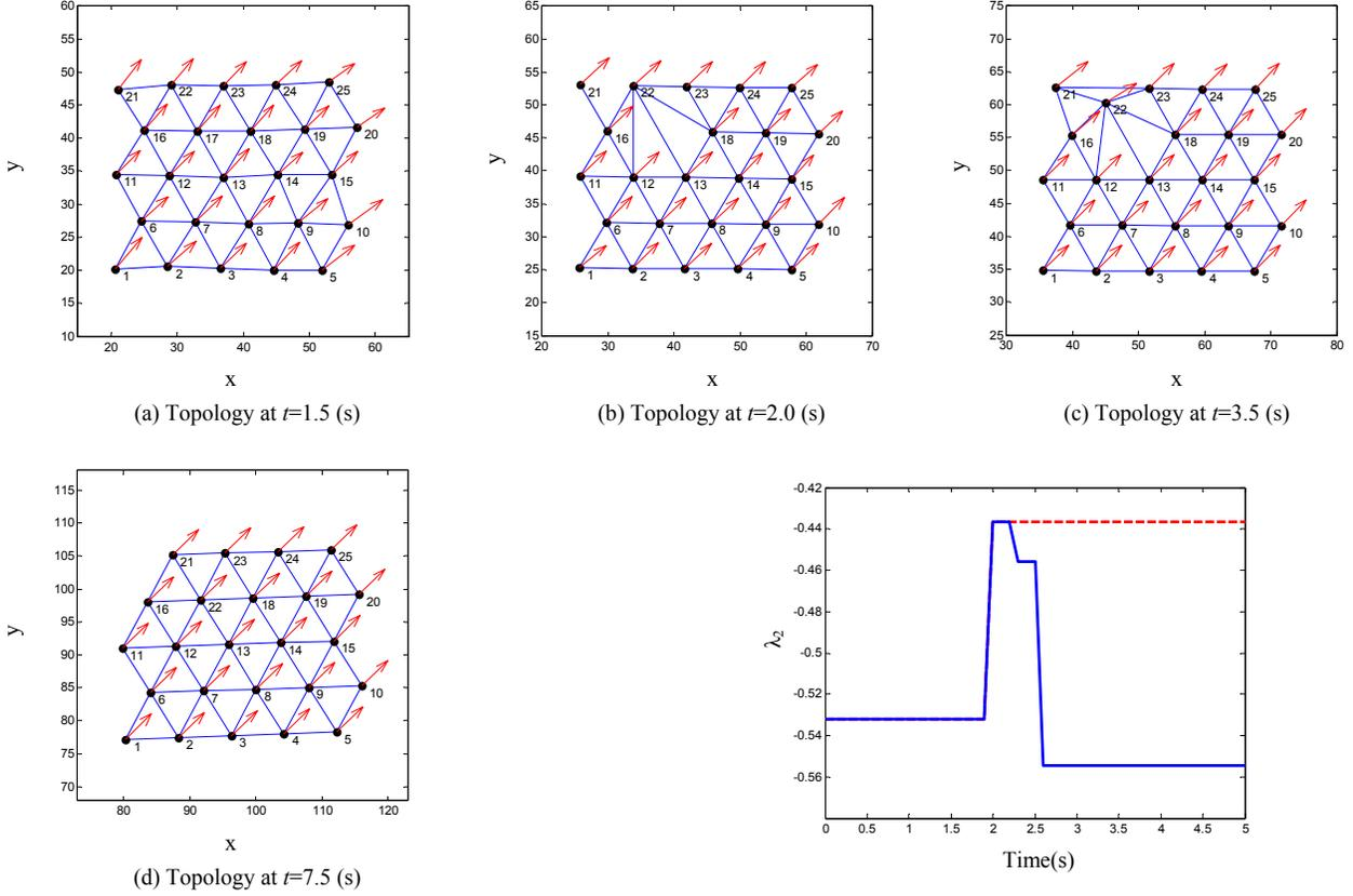
Fig. 2 Simulation results of self-healing for one failed robot.
