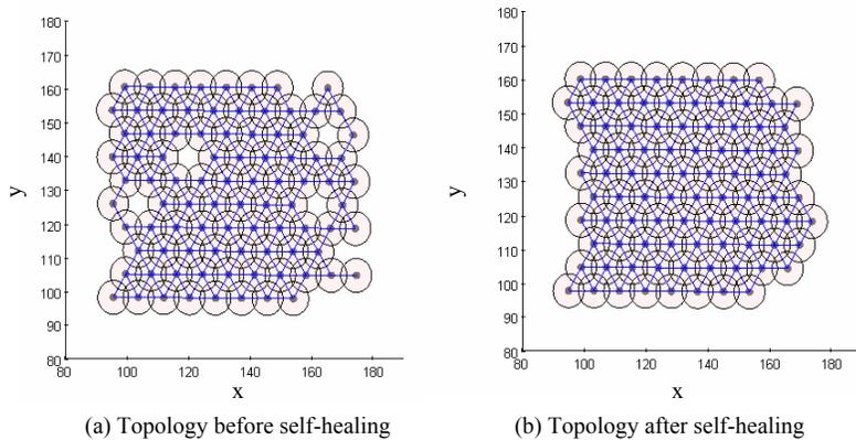
Fig. 4 Simulation results of self-healing for failed robots.
