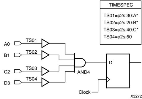
**Figure 18. TIMESPEC Placement Where Some Specifications are Lost**
