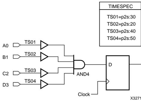
**Figure 17. TIMESPEC Placement Where Some Specifications are Overridden**
