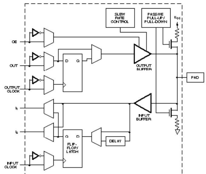
**Figure 8. XC4000 Input/Output Block**
