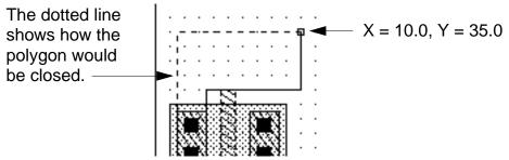
The polygon is 1 micron outside of the p-transistor.
