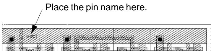
The name *vdd!* disappears from the Create Shape Pin form. The first name listed is now *gnd!* (the ground pin).
