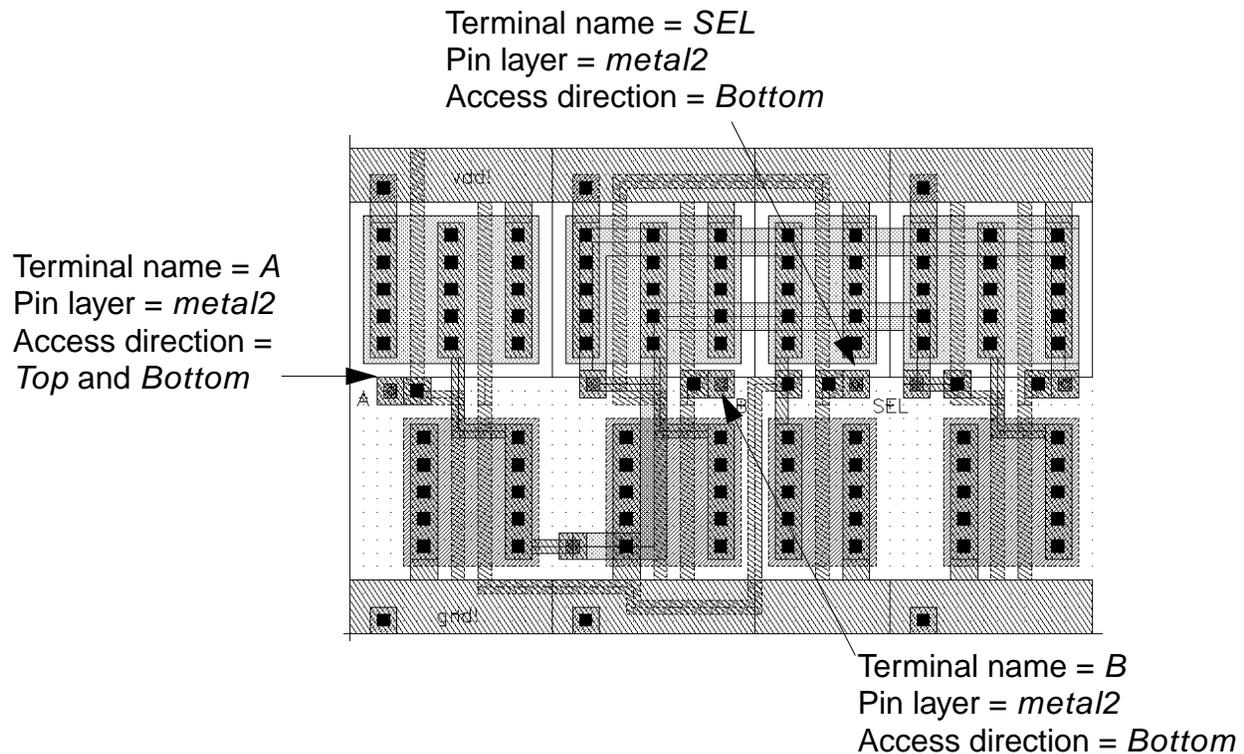
After you create the pins shown in the illustration, the pin form now shows only one pin to create: the Y pin for the multiplexer output.
