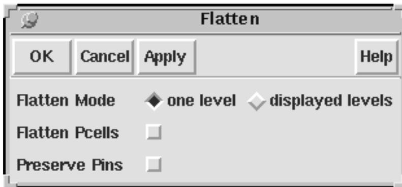
The Flatten form appears. You need to move the contents of *mux2\_connect* up just one level (from level 1 to level 0). The default form settings are set correctly.
