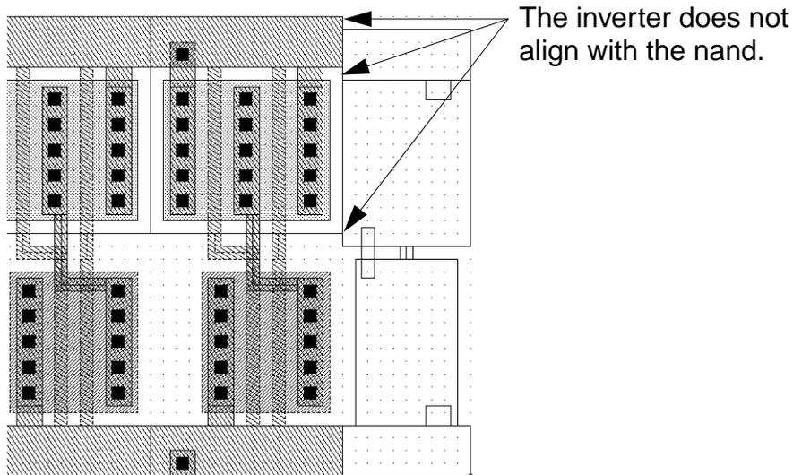
The inverter is not aligned properly with the nands. You correct this error in the following section.
