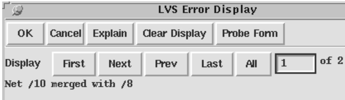
**Note:** LVS assigns numbers to the unlabeled nets. The numbers it assigns to your nets might not be identical to the net numbers shown above. Substitute the numbers on your LVS Error Display form in the following instructions.
