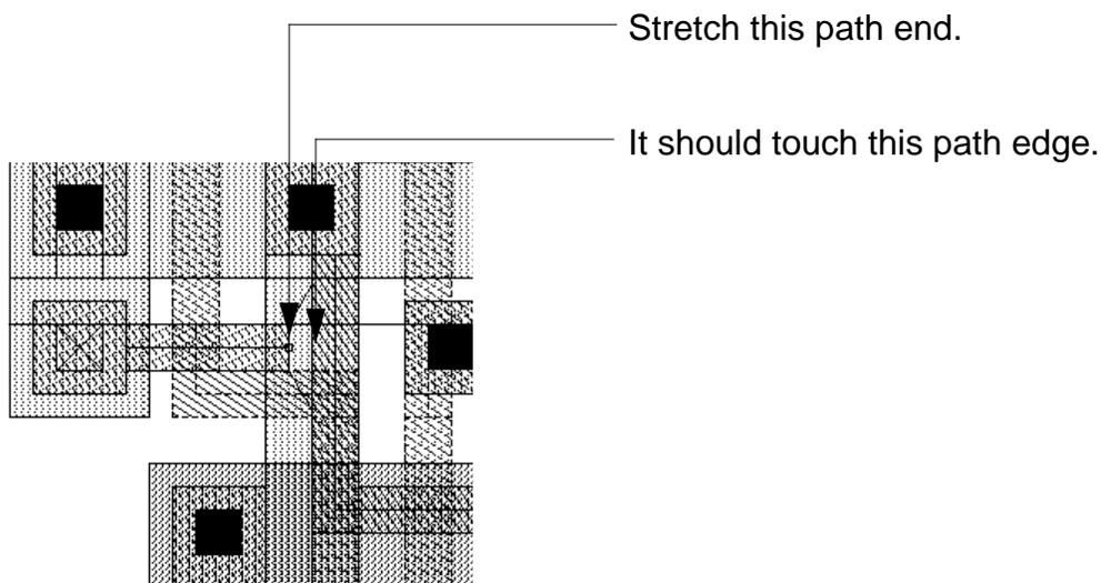
3. To stop the *Stretch* command, press the `Escape` key.
