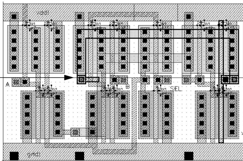
4. In the Probing form, change *Probing Method* to *cross probe*. If you are running Analog Artist, change the Probing Method to *cross probe matched*.
