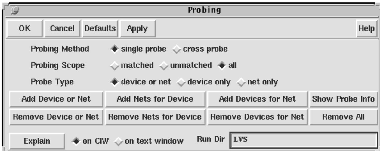
By default, the form is set to perform a single probe. You first probe the extracted view for net 10.
