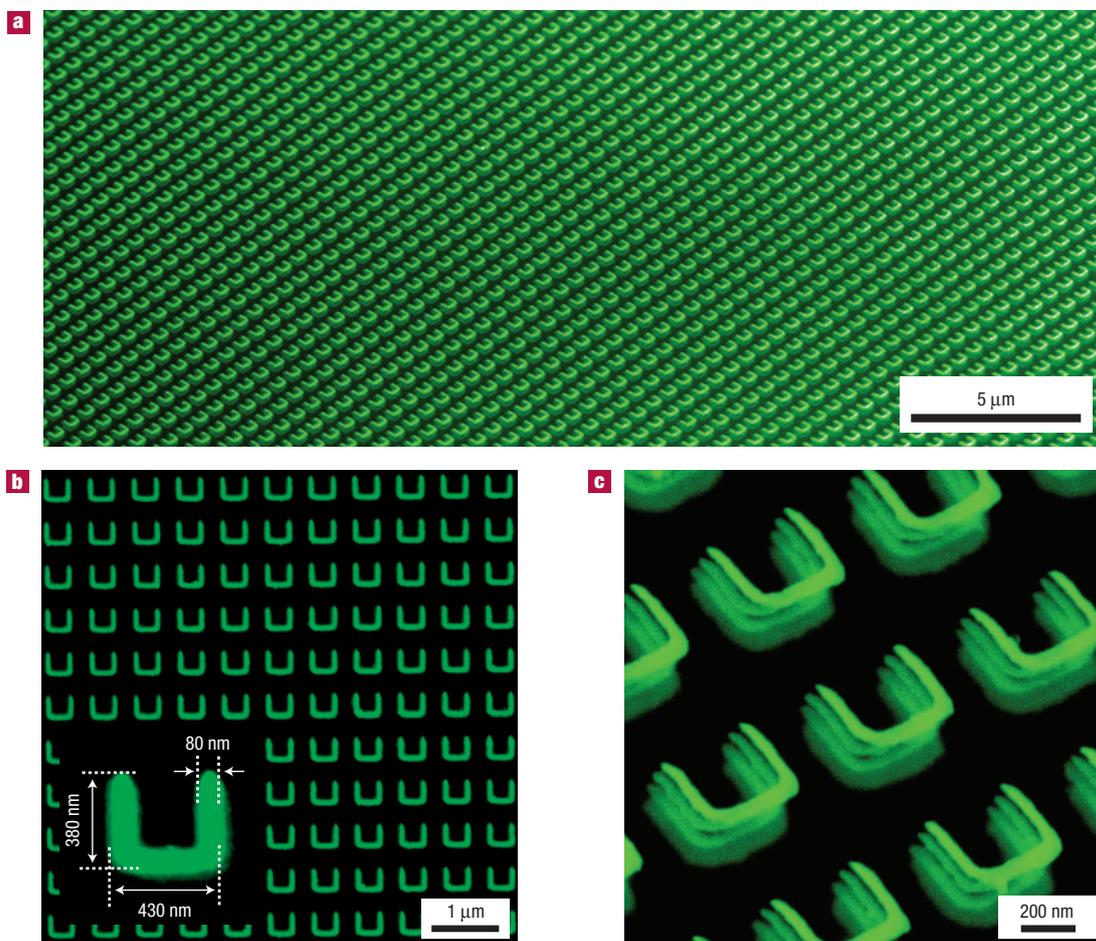
**Figure 2** Field-emission scanning electron microscopy images of the four-layer SRR structure. **a**, Oblique incidence overview. **b**, Normal view. Inset: Magnified view. **c**, Enlarged oblique view. The lateral alignment is excellent.
