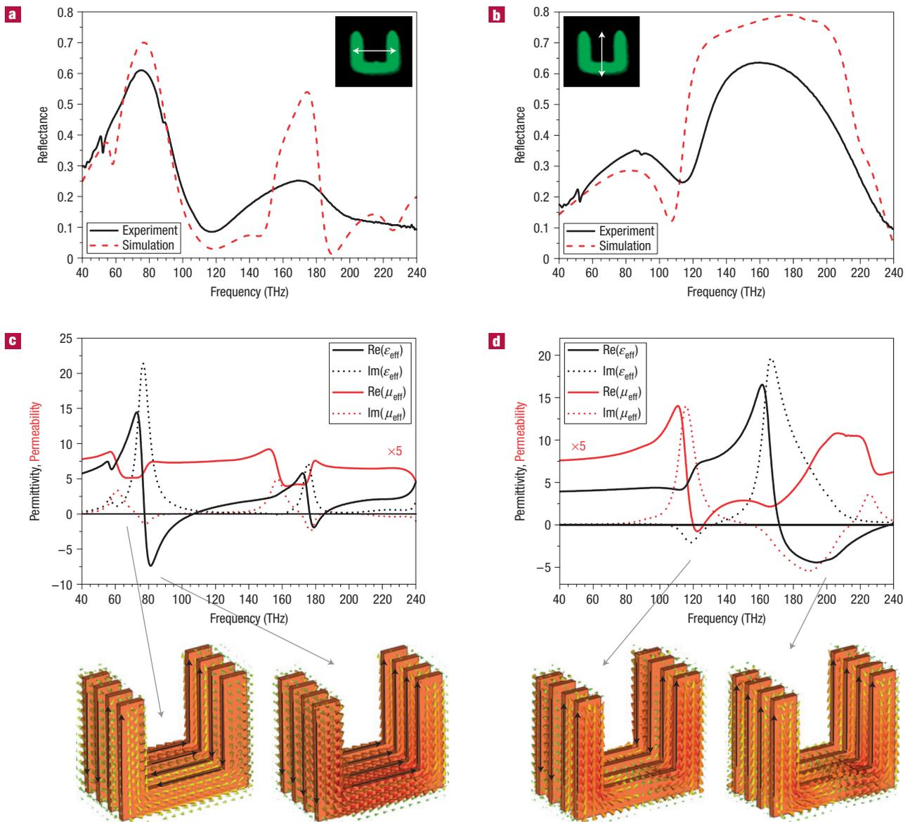
**Figure 3** Experimental measurement and numerical simulation for the four-layer SRR structure. **a–d**, Reflectance spectra, retrieved effective parameters and current distributions at resonances of the four-layer SRR structure for parallel polarization (**a,c**) and perpendicular polarization (**b,d**).
