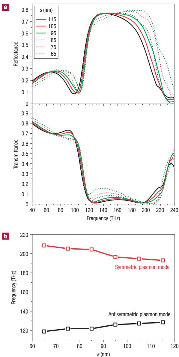
**Figure 4** Optical properties as a function of spacer layer thickness for the four-layer SRR structure. **a**, Simulated reflectance and transmittance spectra as a function of spacer layer thickness for perpendicular polarization (see the inset of Fig. 3b). **b**, Extracted resonant frequencies from **a**.
