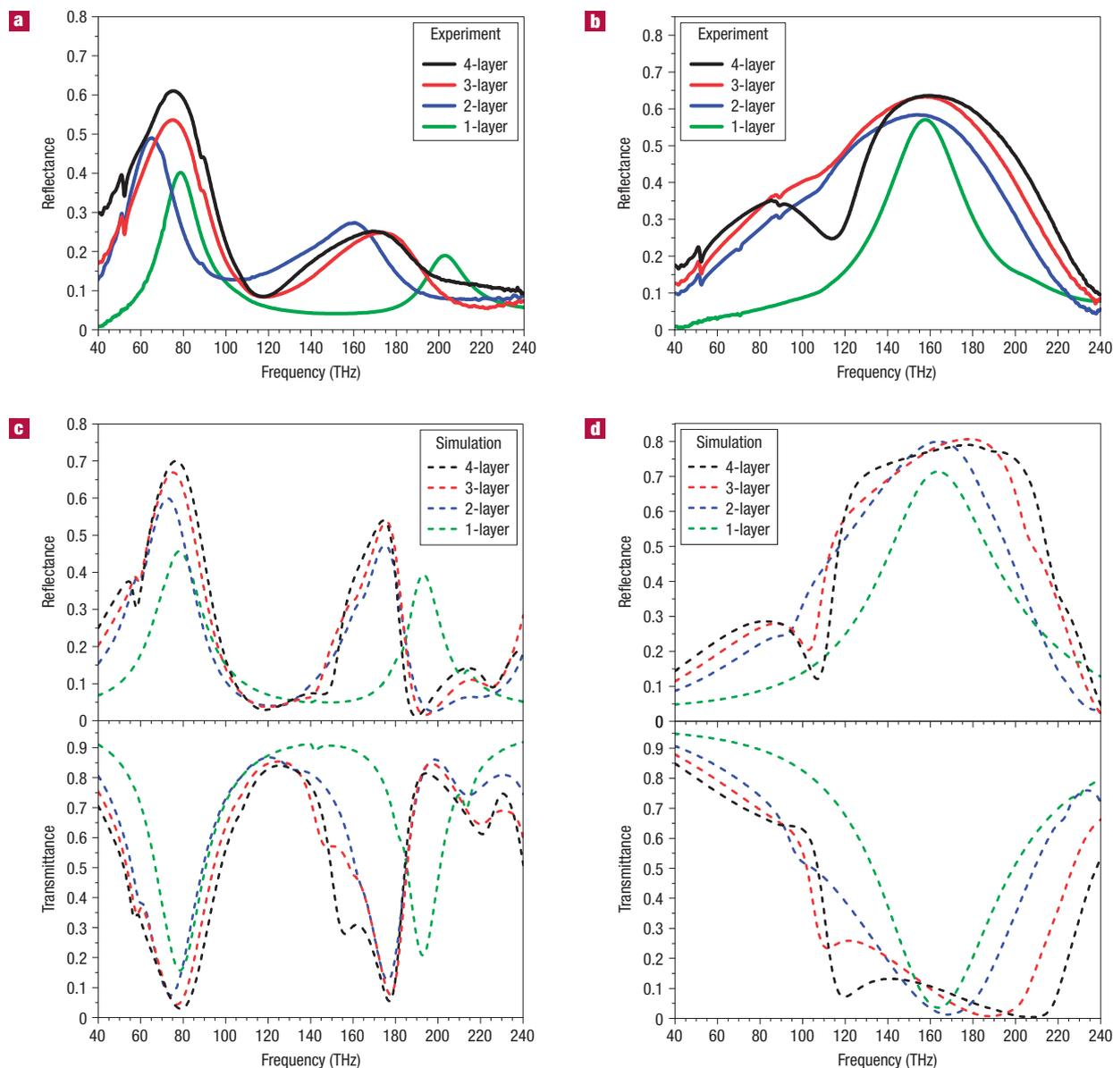
**Figure 5** Evolution of optical spectra with the number of SRR layers. **a–d**, Experimental and simulated reflectance and transmittance spectra for parallel polarization (**a,c**) and perpendicular polarization (**b,d**). The broadening of the resonance with increasing layer number is clearly visible in **d**.
