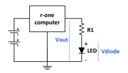
The trick is to use the r-one computer to turn the LED on and off quickly, too quickly for us to see. The flicker fusion rate for human vision is 60hz<sup>1</sup>. This means that anything that happens faster than 60 times a second appears as continuous, smooth motion to us. This is how movies and TV work, and we will use this fact to adjust the brightness of our LED.
