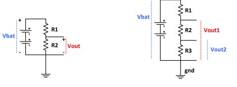
a.  $R1 = 10k\Omega$ ,  $R2 = 10k\Omega$ b.  $R1 = 10k\Omega$ ,  $R2 = 100\Omega$ c.  $R1 = 10k\Omega$ ,  $R2 = 10meg\Omega(1 \times 10^7\Omega)$
