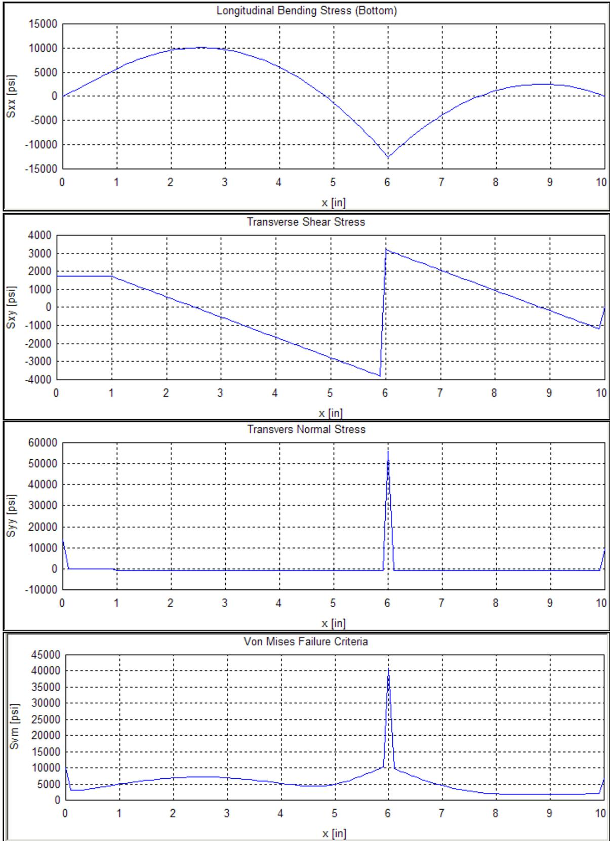
Figure 15 Corresponding stresses for example three point beam
