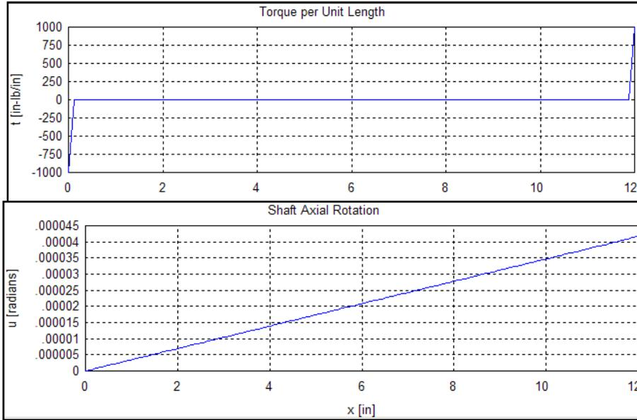
**Figure 8 Shaft with two equal and opposite end torques**
