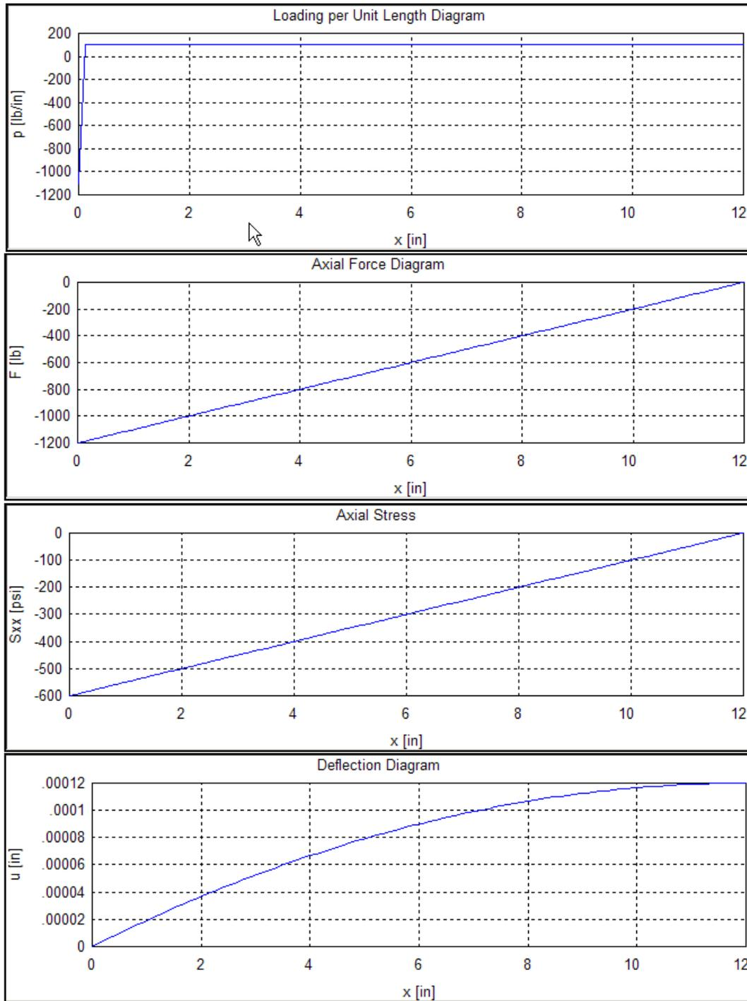
Figure 6 Graphs for fixed-free axial bar hanging under its own weight
