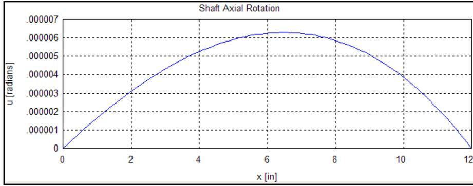
Figure 10 Rotations of fixed-fixed shaft with variable distributed torque
