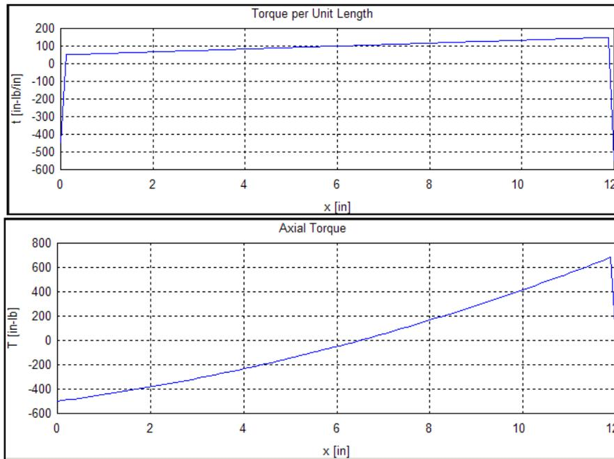
**Figure 9 Fixed-fixed shaft with trapezoidal distributed torque per unit length**
