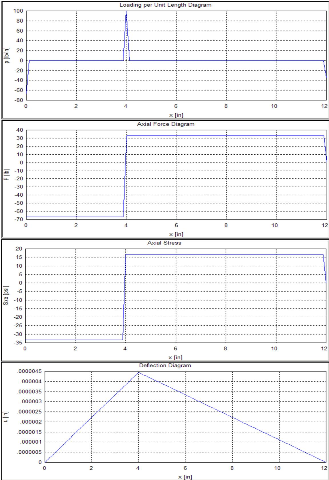
Figure 4 Graphs for fixed-fixed bar with a point load
