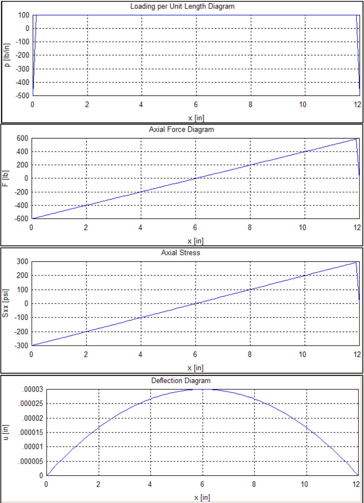
Figure 5 Graphs of a fixed-fixed bar with constant load per unit length
