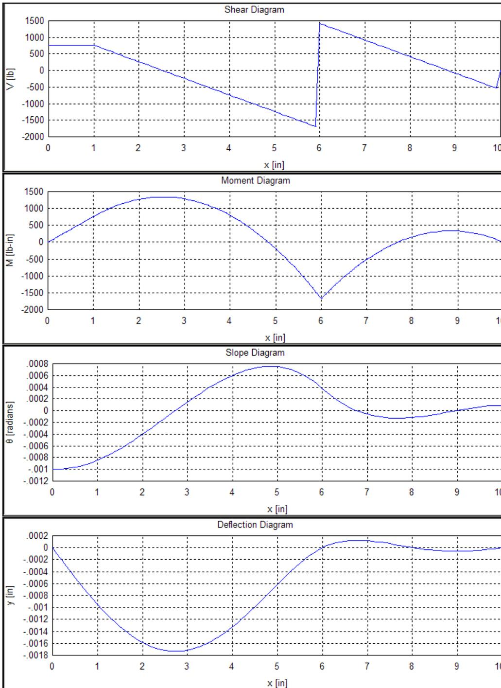
Figure 14 Example shear, moment, slope and deflection of three point beam
