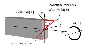
$$W_{I} = \iiint \sigma \cdot \varepsilon \, dx dy dz = \iiint \frac{M(x)y}{I_{z}} \frac{M(x)y}{EI_{z}} dx dy dz$$
