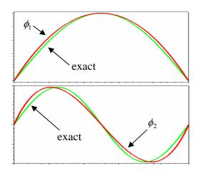
It is clear that the accuracy of the FE approach is dependant the displacement shape function. This is true if only one element is employed. To improve accuracy there are two alternate strategies you could adopt. (a) increase order of polynomial displacement shape function; or (b) use more that one element. (b) is the most commonly adopted strategy and is the basis of the finite element method<sup>4</sup>
