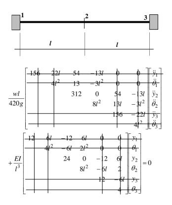
(17) and (31) are substituted into equation (j) to gives the above. By applying support restraints i.e.  $v_1 = v_3 = \theta_1 = \theta_3 = 0$  these degrees of freedom are removed from the problem.
