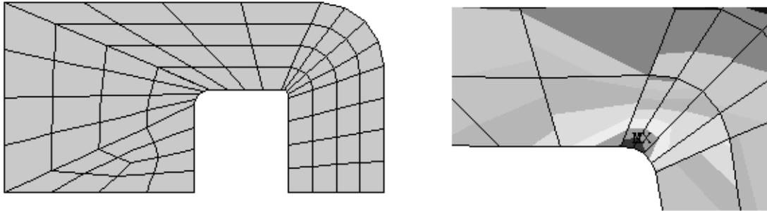
**Figure 2-35** Mapped mesh and von Mises results.
