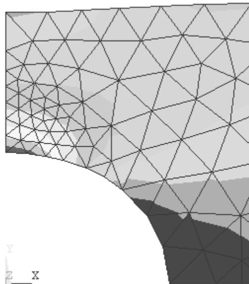
**Figure 2-20** SX stress detail contour after mesh refinement.
