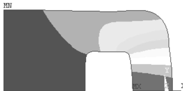
**Figure 2-31** UX displacements.
