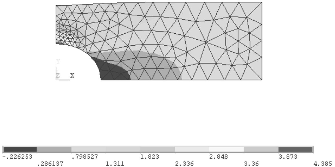
**Figure 2-19** SX stress contour after mesh refinement.
