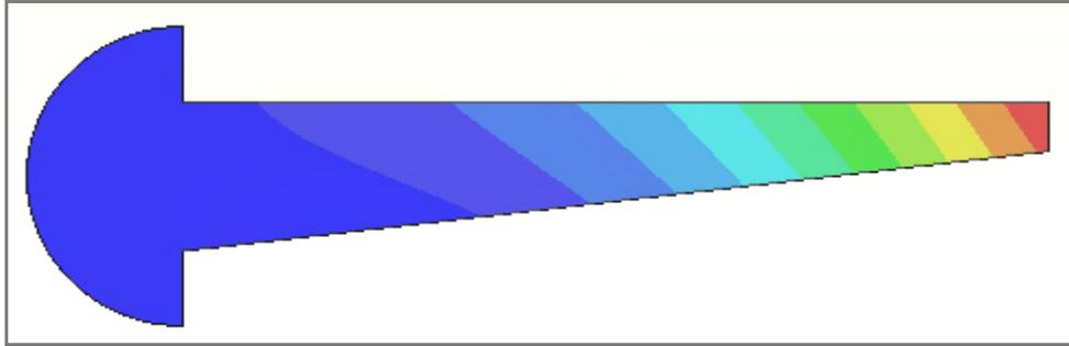
Figure 12-6 Relative buckling mode displacement values (normal to surface)
