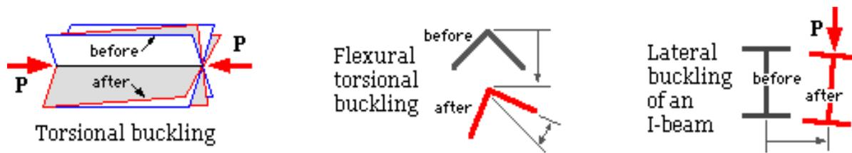
Figure 12-4 Some sample buckling shapes
