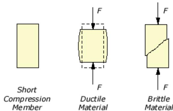
Figure 12-1 Short columns fail due to material failure
