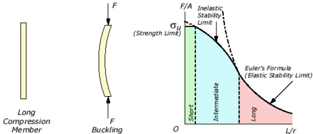
Figure 12-2 Long columns fail due to instability
