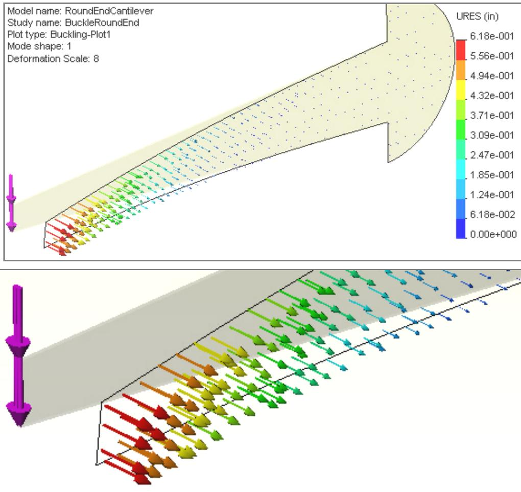
Figure 12-7 Relative lateral buckling mode displacement vectors
