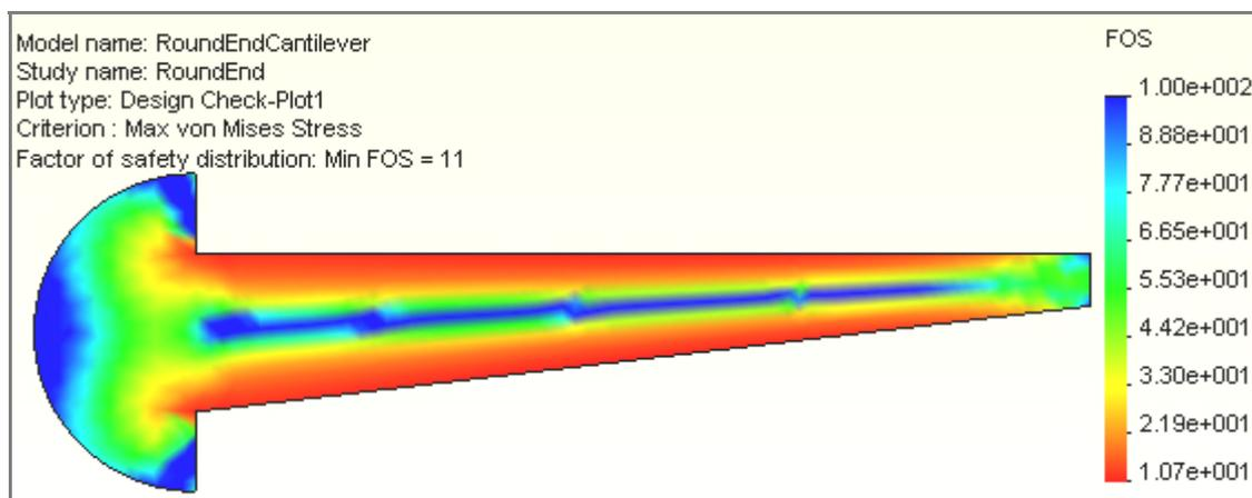
Figure 12-5 Original material factor of safety in bending
