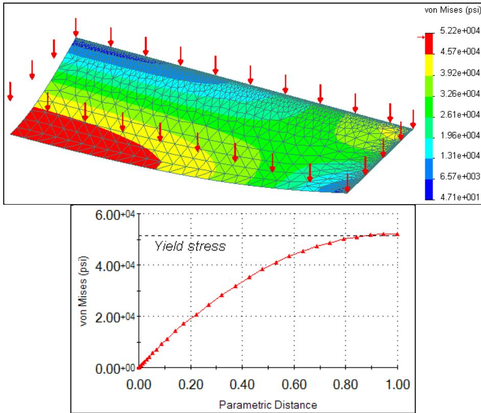
Figure 8-7 Von Mises stress in quarter symmetry plate and its short symmetry side
