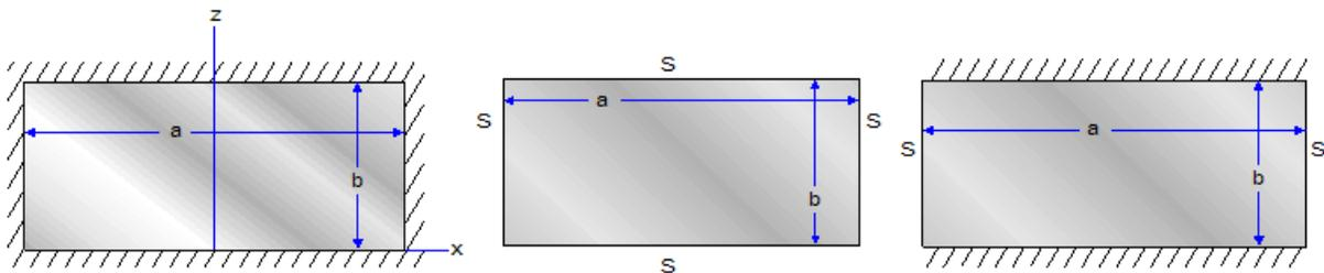
Figure 8-1 Some typical boundary condition options on rectangular plates
