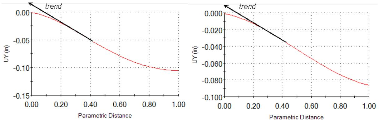
**Figure 8-6 Deflection along from corner to corner (left) and to mid-side**
