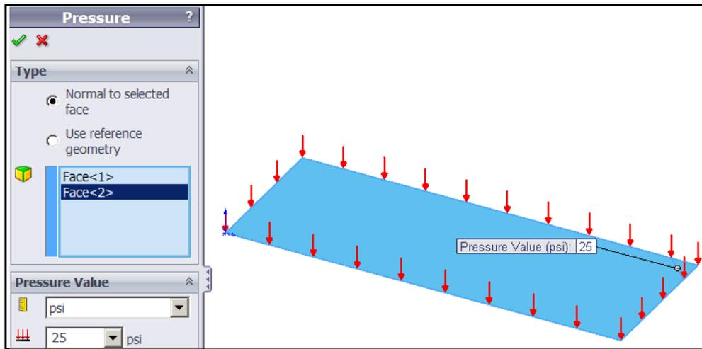
Figure 8-3 Constant normal pressure load on the plate
