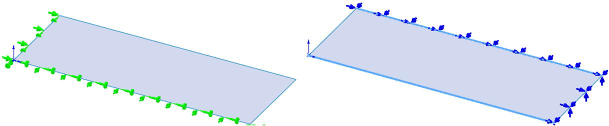
Figure 8-2 Symmetry (left) and simple supported plate restraints
