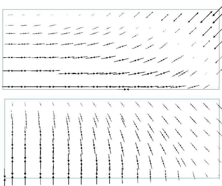
Figure 8-8 The principal stresses P1 and P3 on the top of the quarter symmetry plate
