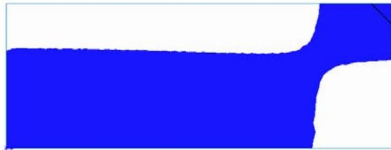
Figure 8-9 Main material load path region of the plate
