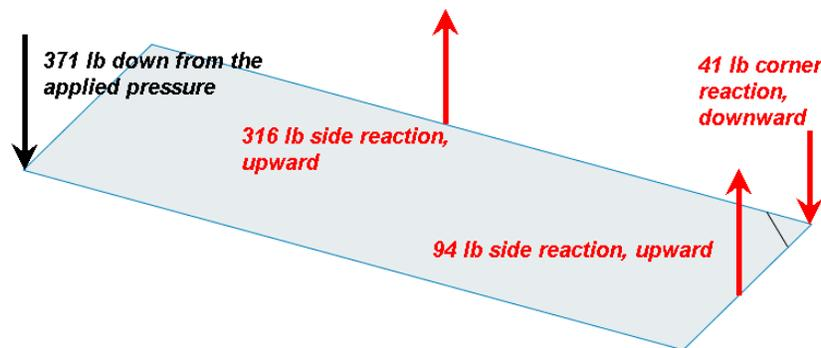
Figure 8-10 Approximate resultant applied force and reaction forces on the plate
