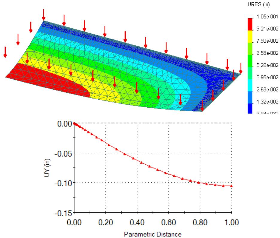
**Figure 8-5 Deflections of the quarter symmetry plate, and its short edge**
