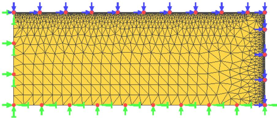
Figure 8-4 Refined edge mesh for a quarter symmetry rectangular plate
