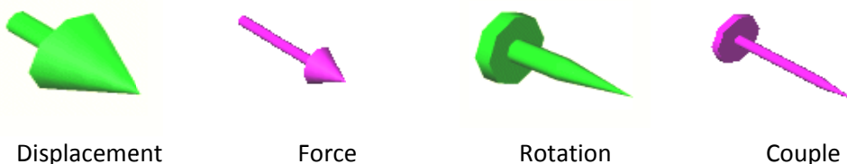
Figure 3-11 Single component symbols for restraints (fixtures) and loads
