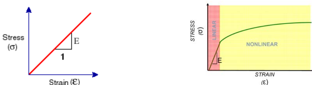
Figure 3-3 Hooke's Law for linear stress-strain, \boldsymbol{\sigma} = \mathbf{E} \boldsymbol{\epsilon}
