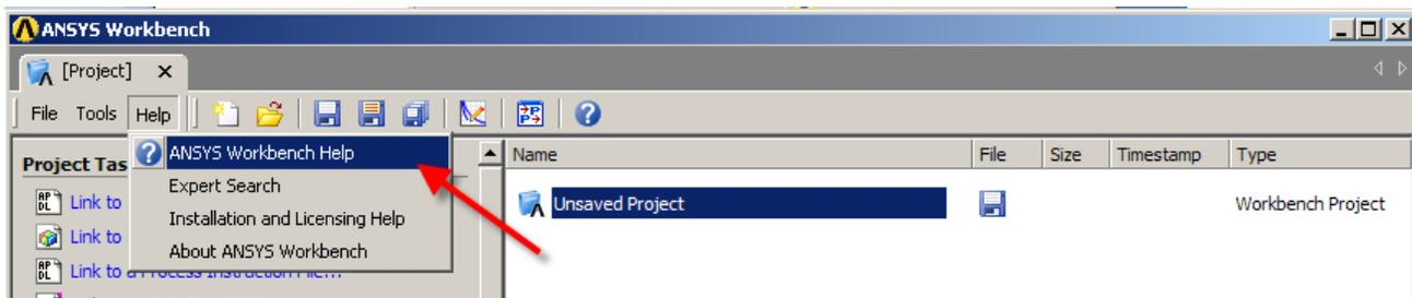
4. Look for “**Release 11.0 Documentation for ANSYS Workbench**”->“**CFX-Mesh Help**”->“**CFX-Mesh Tutorials**” in the “**Contents**” tab on the left.
