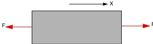
Numerical approximations can lead to rigid body motion in the X direction even when the applied forces are balanced.
