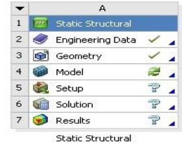
2. From the Geometry cell, RMB and “Import Geometry > Browse”. Import the file “Pump\_assy\_3.stp”.
