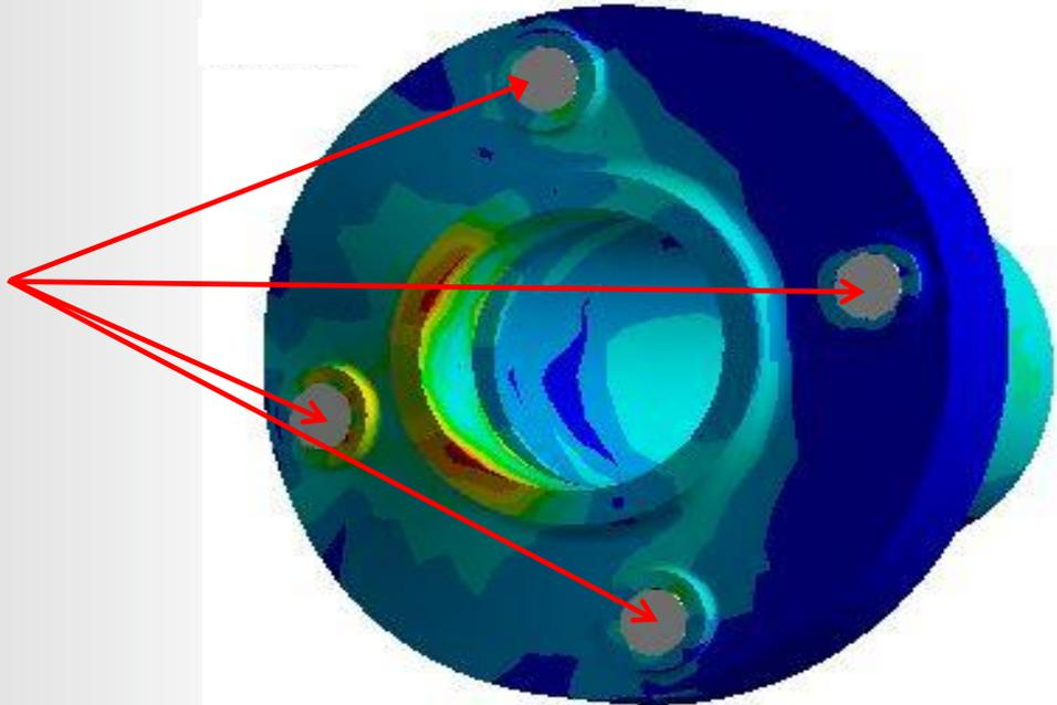
By turning on Auto Scale from the context menu (magnifying displacements) you can see the tendency for the flange to separate due to the remote force.
