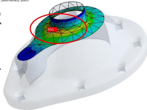
As the plot shows the potential problem areas are around the blend on the top of housing. An efficient approach to investigate these areas in more detail is to create a submodel of this part of the geometry. In this example we have used ANSYS DesignModeler geometry application to slice out a portion of the model which we will use next.
